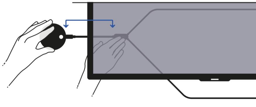
**Keep the Aircord straight** and stick the cable splitter to a surface behind the TV.
