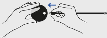
**Hold Airtame 2** onto the magnetic wall mount while plugging in the USB-C cable.
