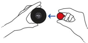
Fix the magnetic wall mount on the back of the Airtame 2
